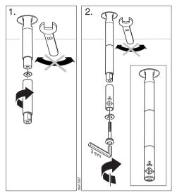
The joystick can be extended for an easier reach.
